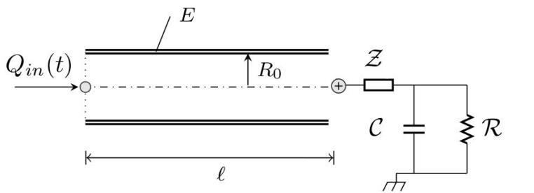
Single vessel + capillary bed model
